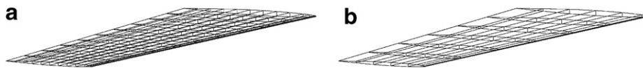
Fig. 8. Fine and coarse FE model of the AGARD 445.6 wing: (a) fine FE model and (b) coarse FE model.
